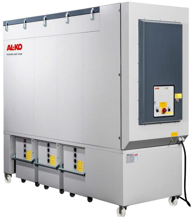
The integrated pre-separator protects the filter bags from direct impact and achieves a high degree of pre-separation through decompression of the airflow. Thus, the greatly reduced impact on the filter significantly increases the endurance and service life of the filter bags.
