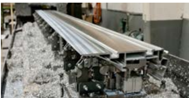
Milling of sliding table surface
