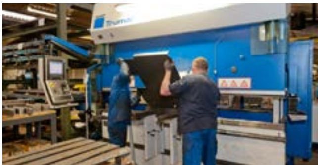
Computer assisted steel plate bending
