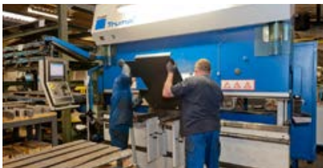
Computer assisted steel plate bending
