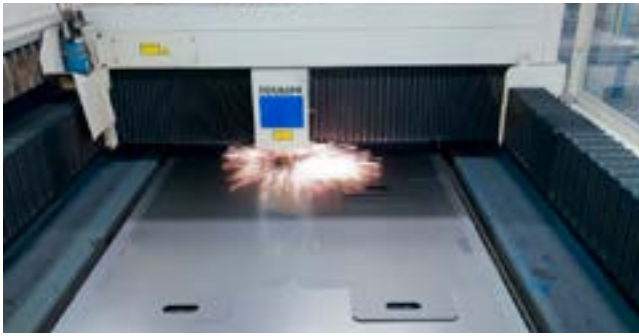
Steel plate laser cutting
