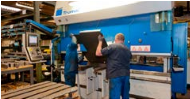
Computer assisted steel plate bending
